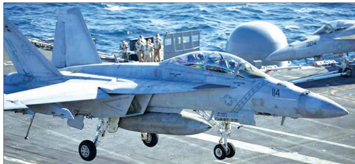
A US Navy F/A-18 Super Hornet fighter lands onto the deck of the USS Ronald Reagan, a Nimitz-class nuclear-powered super carrier, in the West Sea, South Korea on 29 October 2015. PHOTO: REUTERS
