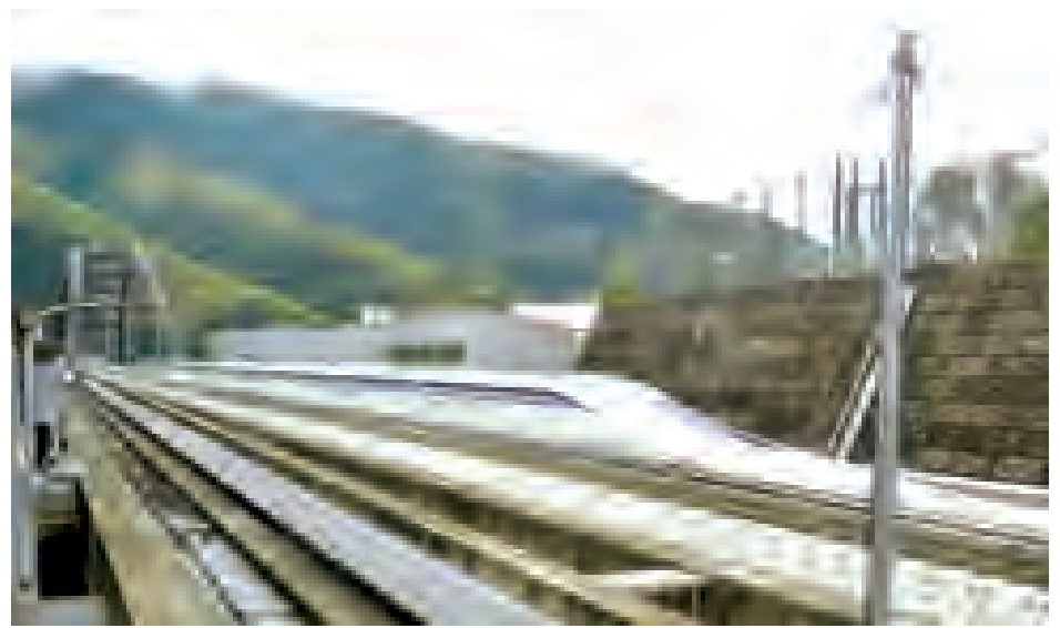
Photo shows a magnetically levitated train operated by Central Japan Railway Co making a test run on an experimental track in the city of Tsuru, Yamanashi Prefecture, central Japan, on 21 April, 2015. The train set a world speed record of 603 kilometres per hour during a manned test run, breaking its own previous record of 590 kph.—KYODO NEWS
