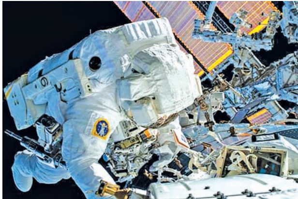
NASA astronaut Terry Virts works to complete a cable routing task near the forward facing port of the Harmony module on the International Space Station, on 21 Feb, 2015.—REUTERS
