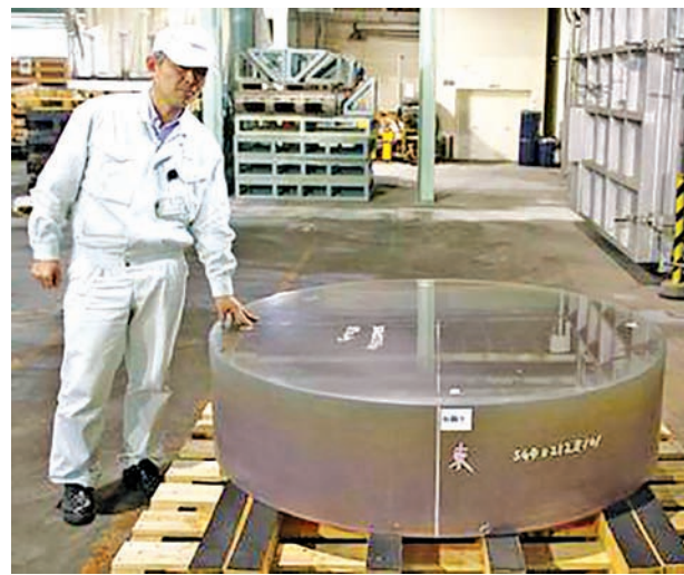
Glass craftsman Hiroyuki Minamikawa stands with an optical lens featuring zero thermal expansion in Sagami-hara, southwest of Tokyo, on 17 Dec, 2014. The lens will be one of 492 pieces constituting the main mirror for the world's biggest telescope called "Thirty Meter Telescope" or TMT set for completion in 2022 on Hawaii Island. —KYODO NEWS
