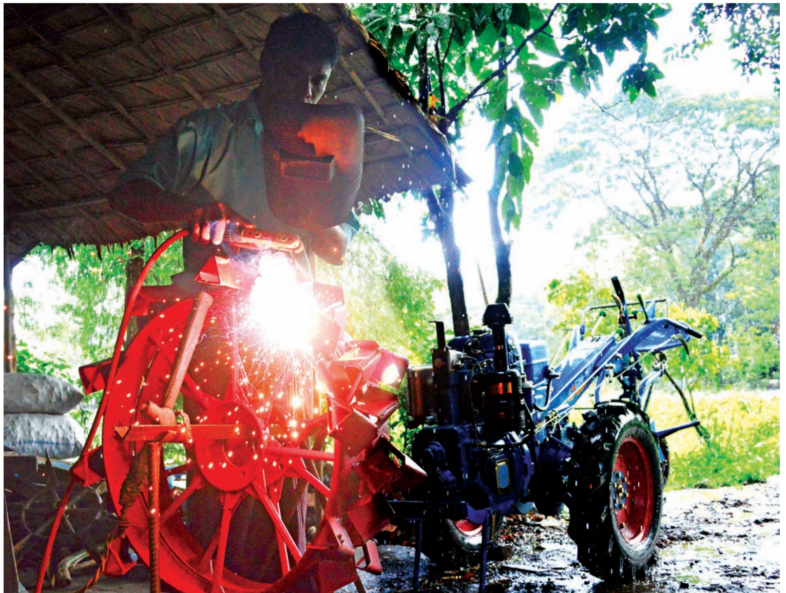
See page 2>> A man make ploughing tool which can be used with a power tiller. PHOTO: AYE MIN SOE
