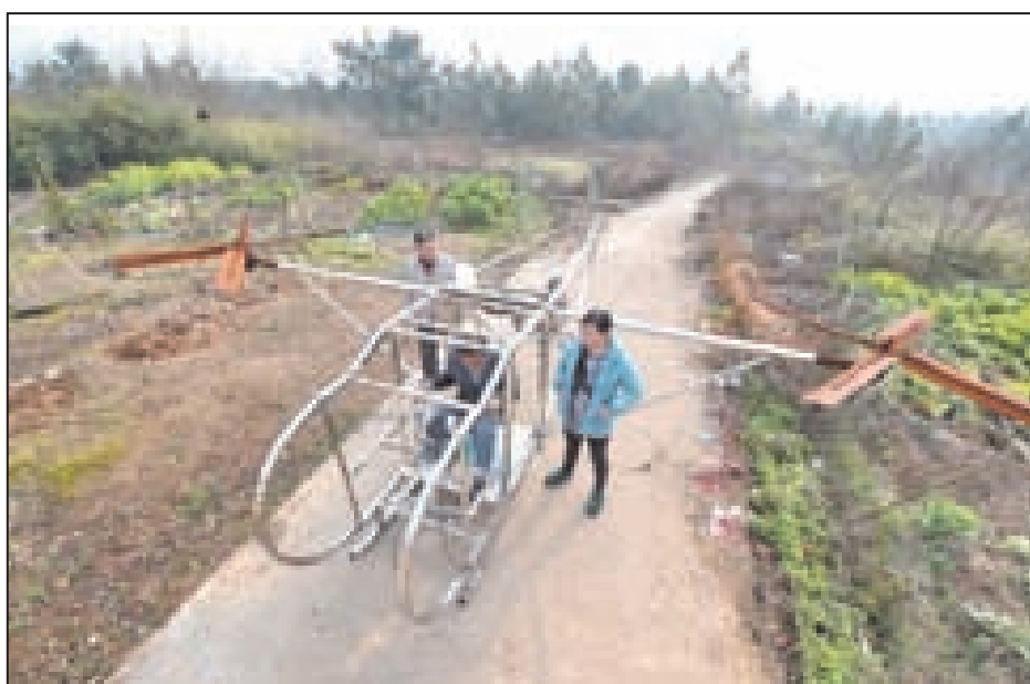
Farmer Li Housheng (C) introduces his flight plan as he sits in his helicopter in Ganzhou Village of Baitang Township in Miluo City, central China's Hunan Province, on 14 March, 2014. Farmer Li Housheng, 52, has started making his twin-rotor helicopter since August 2013. The helicopter has an engine transplanted from an agricultural motorcycle with skeletons made of angle iron and stainless steel tubes. Each rotor is simply a welding of four steel plates. The helicopter's control system including accelerator, clutch and joystick comes from a motorcycle. The helicopter completed a flight test with the fuselage hopping by 40 centimetres from the ground, according to Li. The farmer are now trying to meliorate his helicopter to make his plane as well as his dream to fly higher.
