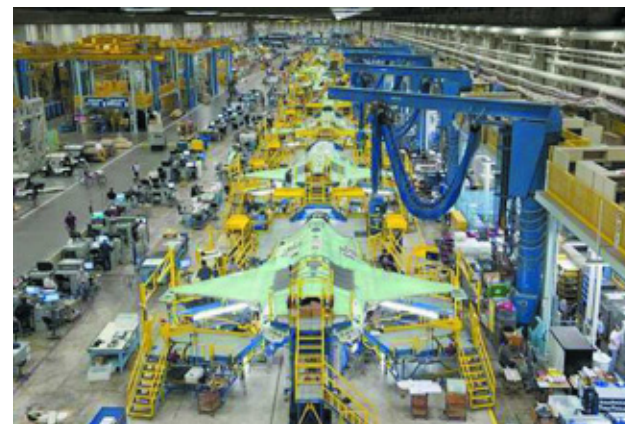
Workers can be seen on the moving line and forward fuselage assembly areas for the F-35 Joint Strike Fighter at Lockheed Martin Corp's factory located in Fort Worth, Texas in this 13 Oct, 2011 handout photo provided by Lockheed Martin.
