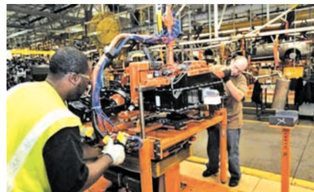
Ford Assembly workers install a battery onto the chassis of a Ford Focus Electric vehicle at the Michigan Assembly Plant in Wayne, Michigan on 7 Nov, 2012.
