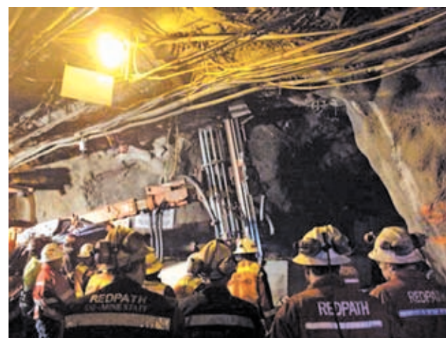
Rescuers use a ground support split set and welded mesh to prevent rockfall during a process rescuing workers still trapped in an underground training class at the Grasberg complex in remote West Papua Province in this 15 May, 2013 picture provided by PT Freeport Indonesia.—REUTERS
