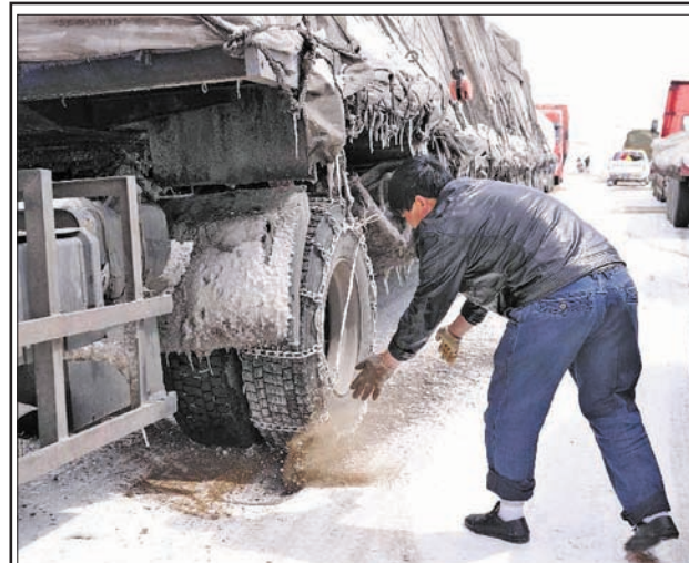
A driver sprinkles salt on the tyres bound with skid-proof chains as vehicles queue to pass the segment of state highway 109 which is covered with snow near Nalong Village in Damxung County, southwest China's Tibet Autonomous Region, on 18 March, 2013. A snowstorm here made an icy road on the segment of state highway 109 near Nalong Village, causing many vehicles truck on the road.— XINHUA
