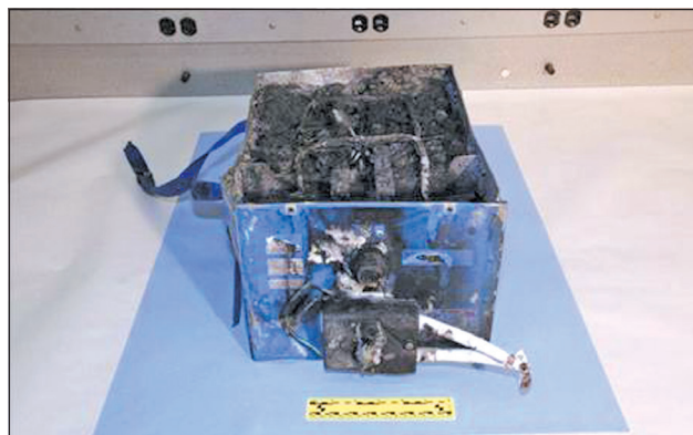
The burnt auxiliary power unit battery removed from a Japan Airlines Boeing 787 Dreamliner jet is seen in this picture provided by the US.—REUTERS
