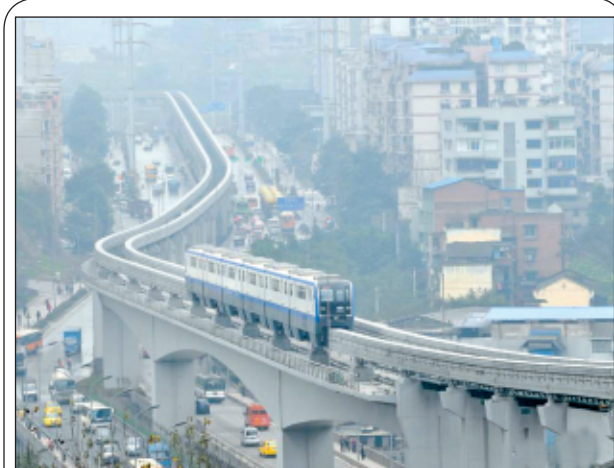
A straddle-type monorail train runs on the No. 3 line of Chongqing's urban railway system in downtown Chongqing, southwest China, on 28 Dec, 2012. The third and last section of Chongqing's No 3 urban railway line was put into trial operation on Friday. The 55.5-kilometre No 3 line connects the southern and northern parts of Chongqing and shortens the travel time in between to 90 minutes.—XINHUA
