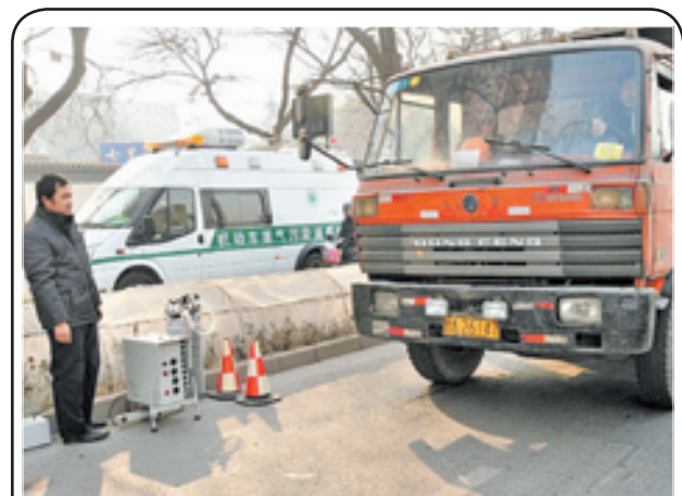
A remote emission test equipment is seen on the street in Lanzhou, capital of northwest China's Gansu Province, on 12 Dec, 2012. Two vehicles with the test system have been put into operation in Lanzhou recently. The system could collect and analyse emission data from a vehicle and record the vehicle number through a remote sensing equipment without interrupting the traffic. XINHUA
