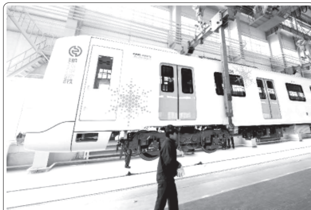
Workers operate a machine to lift the trains for Harbin subway line 1 at the CNR Changchun Railway Vehicle Co, Ltd. in Changchun, capital of northeast China's Jilin Province, on 13 Oct, 2012. The new type of subway trains, which can offer continuous services in extremely cold areas with the lowest temperature of minus 38 degrees Celsius. — XINHUA
