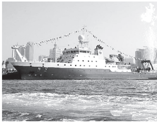
Photo taken on 29 Sept, 2012 shows the comprehensive research vessel, the Kexue ( Science ), in Qingdao, east China's Shandong Province. The 99.6-metre-long and 17.8-metre wide ship was put into service on Saturday. Powered by a podded electric propulsion system, the Kexue consumes less power, creates less noise and vibration, and is able to move at continuously varying speeds of up to 15 knots.—XINHUA
