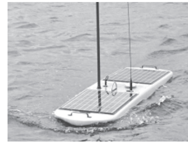
A Wave Glider, a floating platform of sensors with an underwater stabilizer, is seen in this undated handout photo courtesy of Liquid Robotics. REUTERS
