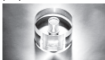
A simple crystal called doped p-terphenyl removes the need for much of masers' complexity.
