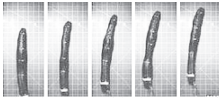
The Meshworm moves itself along by squeezing each of its segments in turn.—INTERNET
