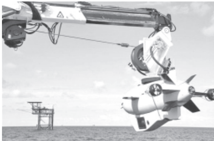
Developed by Lockheed Martin, a 10-foot unmanned submarine named Marlin using sonar and other technologies, is seen in this handout photo taken in the Gulf of Mexico, on 19 July, 2012.— REUTERS
