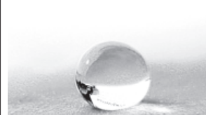
"Hydrophobic" surfaces repel water and grime but can be limited by short lifetimes. INTERNET
