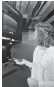
In this 5 June, 1984, file photo, a woman in Chicago demonstrates Atari’s new game, Mind Link, which utilizes a headband that picks up electrical impulse from the movement of the forehead and transmits them to a receiver attached to a video game or home computer console.
