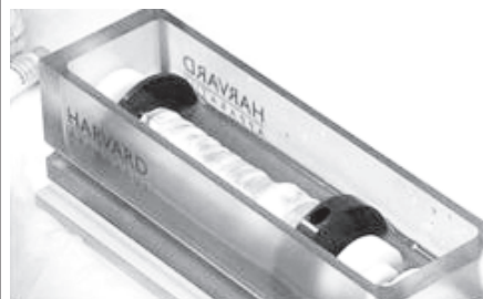
Harvard Bioscience "InBreath" Bioreactor with synthetic laryngotracheal scaffold seeded with patient's own cells. —INTERNET
