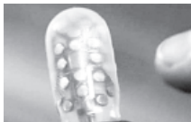
Like the human finger, the BioTac sensor has a soft, flexible skin over a liquid filling.—INTERNET
