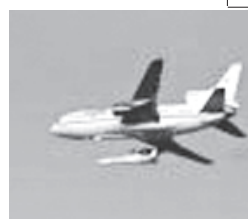
The Orbital Science Corporation’s “Stargazer” plane is shown releasing its Pegasus rocket. NASA’s NuSTAR will also launch from a Pegasus carried by the Stargazer plane.
