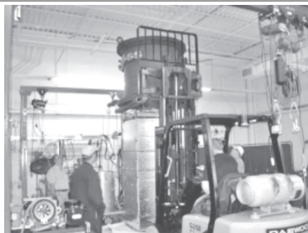
Researchers and staff at UT’s Magnet Development Laboratory prepare the central solenoid mockup for the vacuum pressure impregnation process.—INTERNET
