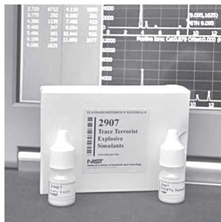
The new NIST reference material can be used to test and validate the ability of machines and methods to detect the explosives’ presence.—INTERNET
