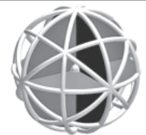
Design for a wind-driven tumbleweed rover.
