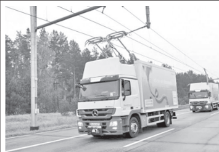
Trucks travel along a test track in Germany, where Siemens is working on its eHighway concept. This system has been proposed to cut pollution on Interstate 710 in LA.—INTERNET
