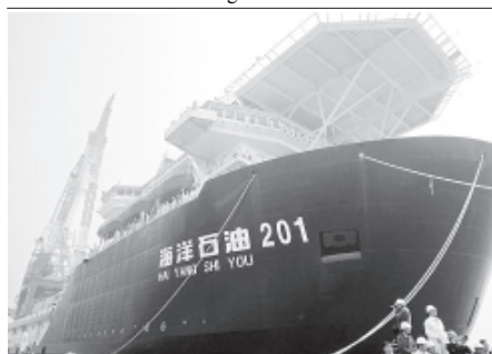
Photo taken on 15 May, 2012 shows the newly-built deepwater pipelay crane vessel "Hai Yang Shi You 201" in Qingdao, a coastal city of east China's Shandong Province. The vessel, with a length of 204.65 metres and width of 39.2 metres, will sail for the South China Sea to conduct pipelay operation in the Liwan 3-1 gasfield.— XINHUA
