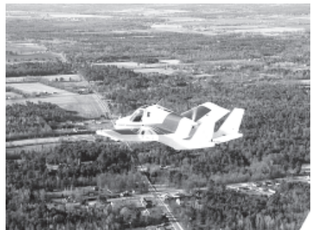
This 23 March, 2012 photo provided by Terrafugia Inc shows the company’s prototype flying car, dubbed the Transition, during its first flight. The vehicle has two seats, four wheels and wings that fold up so it can be driven like a car, and flew at 1,400 feet for eight minutes during the test. Commercial jets fly at 35,000 feet.—INTERNET
