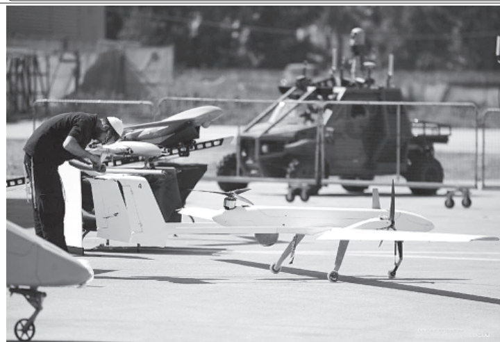
A man adjusts an unmanned aircraft named Panther with a tilt-rotor propeller and a fixed wing vertical takeoff and landing system, which enables runway-free takeoff and landing on an unprepared area, at the campus of Israel Aerospace Industries (IAI), on 22 March, 2012. IAI exhibited its unmanned vehicle production to visitors Thursday. XINHUA
