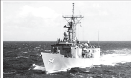
USS Ford (FFG 54) successfully transited from the ship's homeport in Everett, Wash, to San Diego, on 2 March, using 25,000 gallons of a 50/50 algae-derived, hydro-processed algal oil and petroleum F-76 blend in the ships LM 2500 gas turbines.—INTERNET
