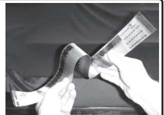
A new sensor was developed for ESA based on super-thin piezoelectric materials that have a special property that converts physical effects like vibration and pressure into minute electric pulses.— INTERNET
