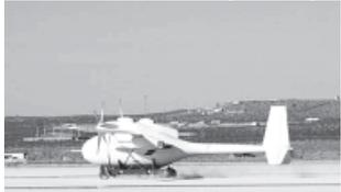
Nestled on its launch cart system, the Phantom Eye traveled some 4,000 feet at speeds of up to 30 mph in a trip that lasted less than two minutes.—INTERNET
