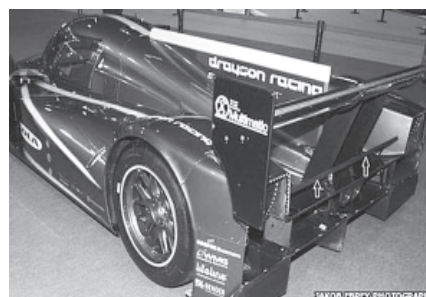
The Lola-Drayson electric car is an opportunity to test the structural batteries which will power some on-board systems. In this image a battery is indicated with yellow arrows.
