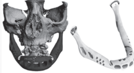
A computer model of the fitted 3D-printed jaw is shown next to an image of the manufactured part.
