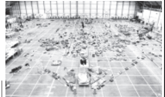
An overview of the Columbia debris reconstruction hangar in 2003 shows the orbiter outline on the floor with some of the 78,760 pieces identified to that date. More than 84,000 pieces of shuttle debris were recovered, some of which is included in a travelling NASA display to stress safety.—INTERNET
