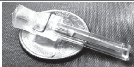
A new type of miniature pressure sensor designed to be implanted in the body is powered by acoustic waves from music.—INTERNET
