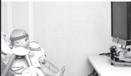
This undated handout photo provided by Florida Atlantic University shows a baby, looking at a monitor, wearing a band that contains a little magnet that the head-tracker, under the monitor uses to determine head position which, in turn, enables the eye tracker to find the eye and the pupil.—INTERNET
