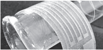
Reactive silver ink is airbrushed onto a thin, stretchy plastic film to make a flexible silver electrode.
