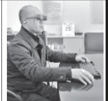
A staff member shows how to use a wearable computer designed by a company in southwest China's Yunnan Province, 6 Jan, 2012. The wearable computer, designed and made by a sci-tech company in Yunnan, includes an eyeglasses-shaped mainframe, a mouse and a folding keyboard.—INTERNET
