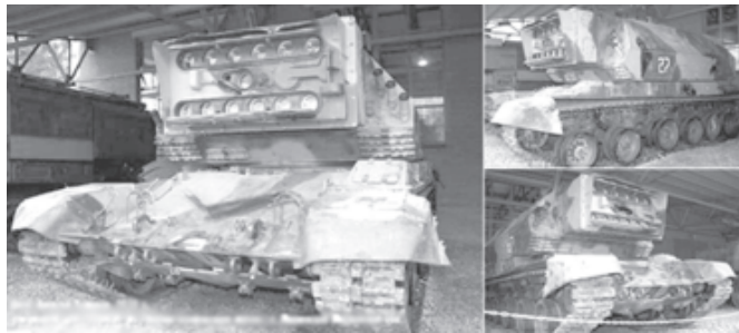
Recently uncovered in a military museum near Moscow, the laser tank can blind pilots and weapons systems by dazzling optical and electronic mechanisms in the battle. — XINHUA
