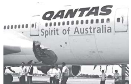
Workers and security personnel stand nearby the Qantas Melbourne-bound Boeing 747 which made an emergency landing in Manila in July 2008 after an explosion in its fuselage. Australian air safety officials have ruled that a "very rare" oxygen bottle explosion was behind the dramatic mid-air blast.
