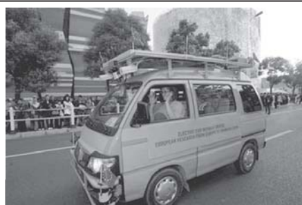
One of two driverless vehicles, equipped with laser scanners and cameras to detect and help avoid obstacles, travels on the Shanghai Expo site to attend the official celebration of their arrival in Shanghai, China, on 28 Oct, 2010.
