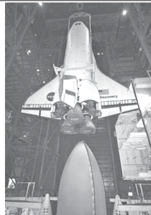
In this image provided by NASA a large yellow, metal sling lowers shuttle Discovery to its external fuel tank and solid rocket boosters on 10 Sept, 2010 before mating to the external fuel tank and twin solid rocket boosters inside the Vehicle Assembly Building, in Cape Canaveral, Fla. INTERNET
