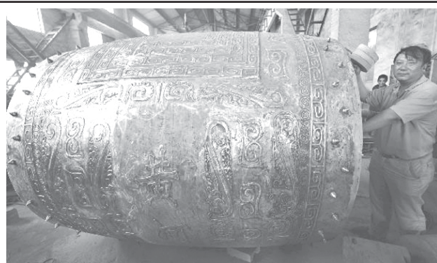
A worker tests the tone of a huge bronze drum which is 2.01 metres in diameter, 2.39 metres in length and 6.3 tons in weight, in Nanjing, capital of east China's Jiangsu Province, on 15 Sept, 2010. —XINHUA
