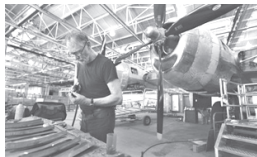
In this photo taken on 14 July, 2010, Bill Wiesner, a retired Boeing machinist, prepares rivets for an engine panel on the Boeing B-29 Superfortress at right that he is helping restore at Boeing Co's historic 'Plant 2' in Seattle.
