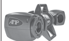
Non-contact 3D Imaging System, the FARO AMP 3D Imager. INTERNET
