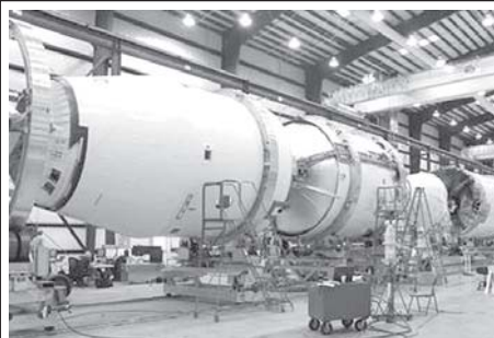
Flight hardware for the inaugural launch of the Falcon 9 rocket undergoes final integration in the hangar at SpaceX's Cape Canaveral launch site in Florida.
