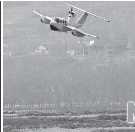
A Wing-In-Ground (WIG) aircraft called "Angel Bird" flies during a trial flight in Nanjing, east China's Jiangsu Province, on 23 April, 2010. The aircraft, developed by Jiangsu Hengchuan Group with independent intellectual property rights, is 10.7 metres wide, 12.6 metres long and 3.5 metres high. XINHUA
