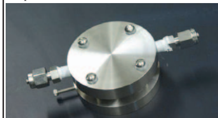
Test battery has inlet and outlet on the sides to provide a flow of air, providing oxygen for the battery's operation.
